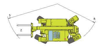
The engine is mounted to the right side of the chassis, ensuring safe, easy access and maintenance from ground level.
