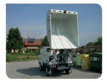
The URBIS 2 & 3 series attachment supplied by TECNOINDUSTRIE MERLO SpA comprises simple rear-loading tanks with tip-up discharge using a specific double-acting cylinder with a single stem. Manual tank loading by operators is facilitated by or tip-up side tailgates on the bodies with stainless steel hinge.
